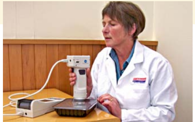
Figure 3. Colour stability measurement with a chromameter
